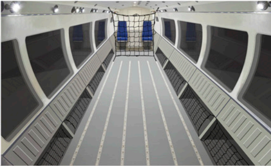
The passenger cabin may be partially or completely converted into the cargo cabin with flat floor if needed
