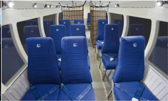
The passenger cabin may be partially or completely converted into the cargo cabin with flat floor if needed
