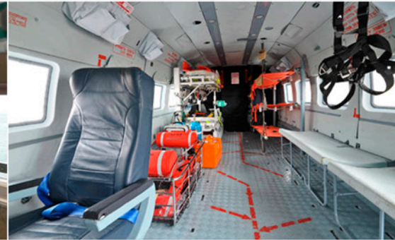
Cabin can be converted into the cargo module for survival equipment delivery
